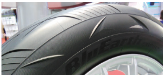
An aerodynamically optimized tire
