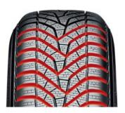
Avoids hydroplaning on slushy or wet surfaces with see-through arrangement.
